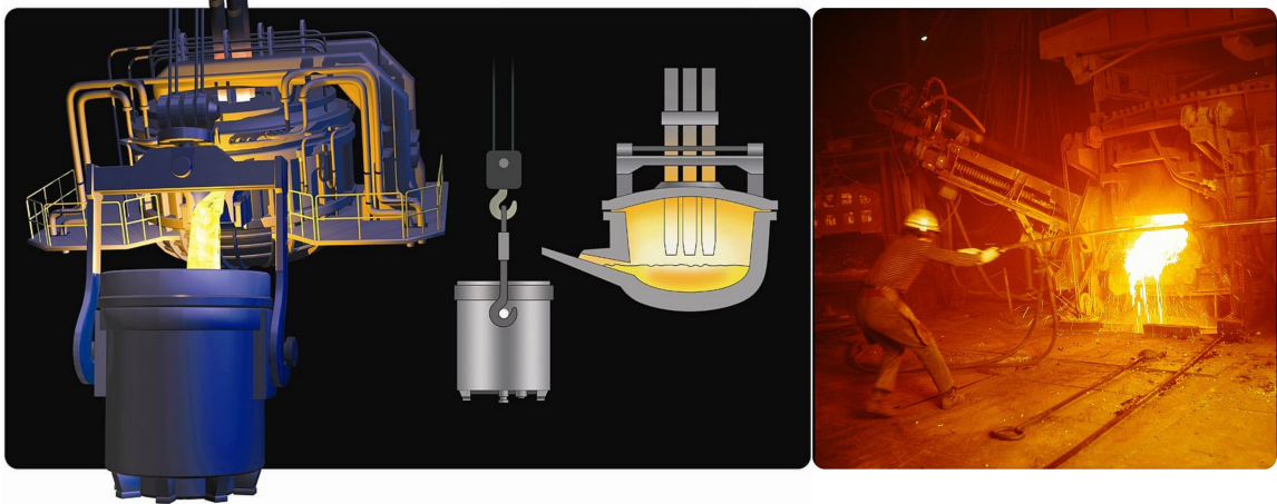
Figure 1.3: Left: Illustration of an Electric Arc Furnace (EAF) during tapping of molten steel into a vessel, and cross-section of a furnace showing the electrodes. Right: a worker manually checks the temperature using a thermocouple attached to a long probe while slag is poured. Image: Deutsche Fotothek (CC BY-SA 3.0 DE).
